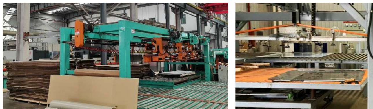
Cold Rolled Continuous Mill Plate 冷轧开平
